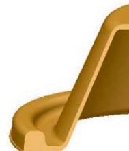
"D" Bead - Over Worse resistance to trapping air Worse flow for less knit lines Better flash location for trimming
