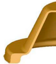
Tear Drop - Under Better resistance to trapping air Better flow for less knit lines Better flash location for trimming
