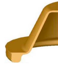
"D" Bead - Under Worse resistance to trapping air Worse flow for less knit lines Worse flash location for trimming
