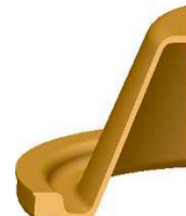
Tear Drop - Over Better resistance to trapping air Better flow for less knit lines Worse flash location for trimming
