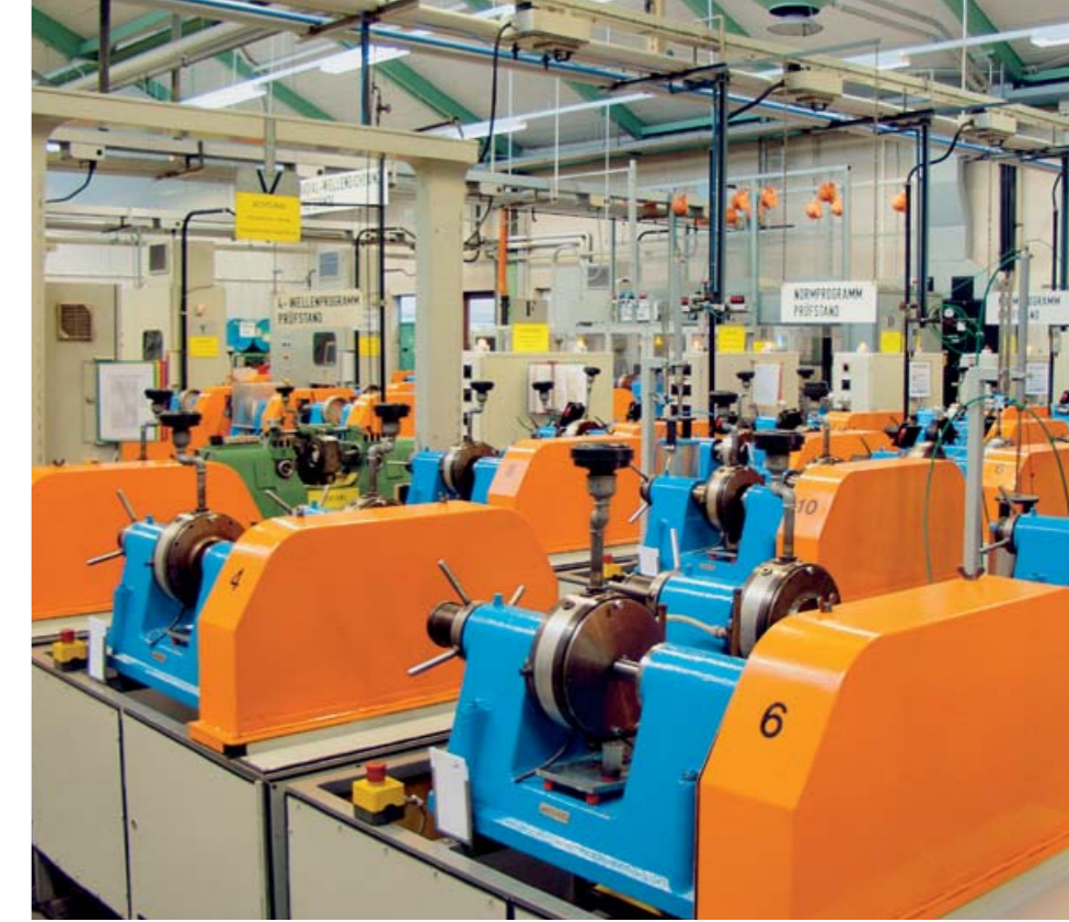
The radial shaft seals test fields at Simrit are equipped with many special installations, as well as standard test benches.
