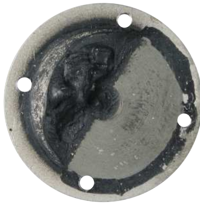
Pulling off of the elastomer from the metal (bonding fault).
