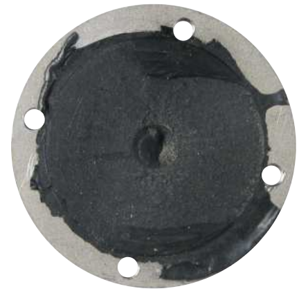
Tear in the elastomer (good rubber-metal-bonding).
