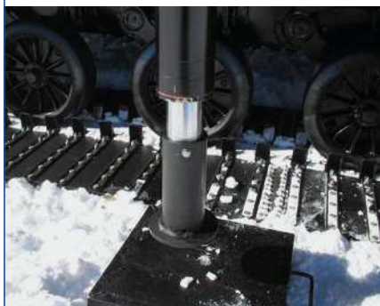
The extension cylinder of the loading crane currently works absolutely leak-free.
